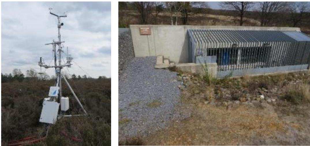
Figure 5: ICOS flux tower (left) and underground technical building (right).
