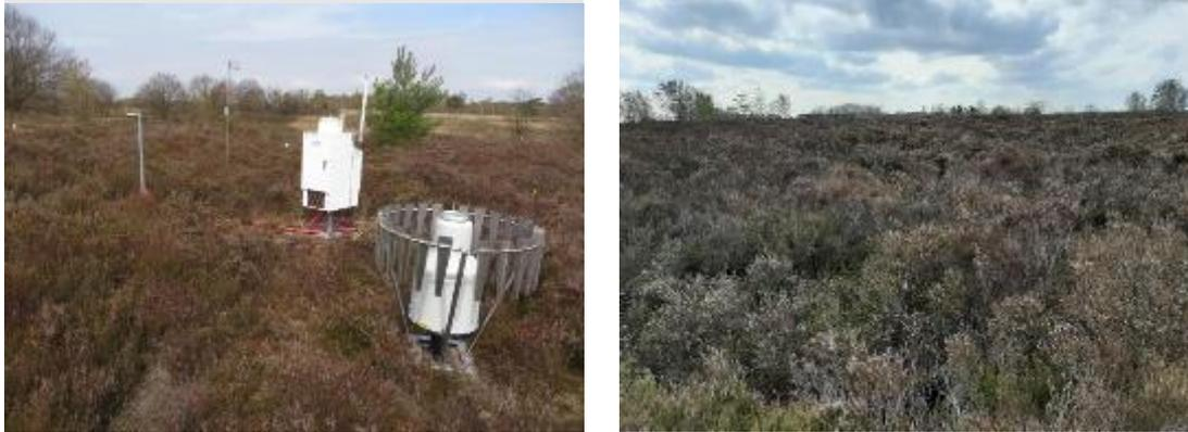
Figure 6: Left photo: VMM monitoring instruments (wet-only sampler, precipitation volume, NH<sub>3</sub> and NO<sub>2</sub> passive samplers). Right photo: View of the heathland to the SW from the COTAG location (April 2021).
