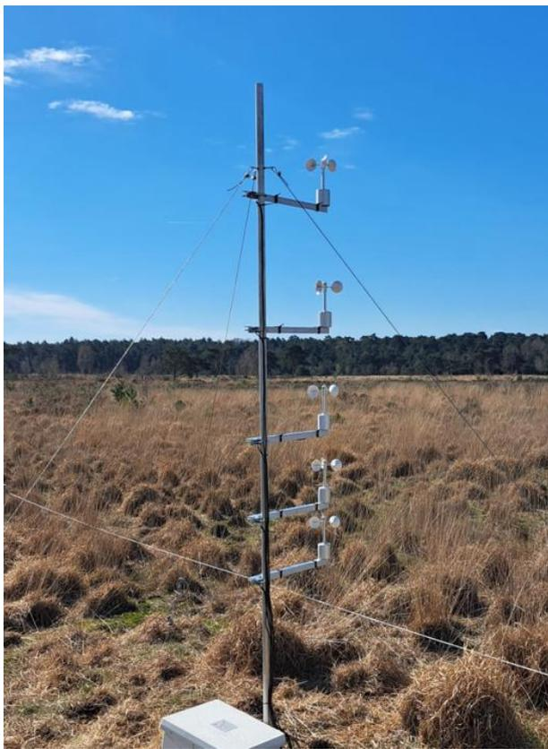
Figure 29: Pole with 5 cup anemometers and datalogger box at Kalmthout.
