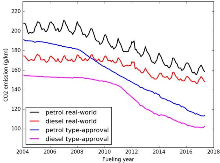
Figure 4-1 There is a clear downward trend in fuel consumption and CO<sub>2</sub> emissions of vehicles, despite the increase in weight, with seasonal variations. These reductions, however, do not follow the trends set out by type-approval results. The real-world CO<sub>2</sub> discrepancy amounts to about 30 g/km, while for diesel vehicles this is reduced by the increase in weight<sup>4</sup>
