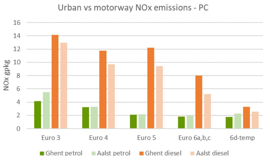
Figure 4-71: Comparison of Ghent (urban) and Aalst (motorway) NOx emissions per Euro class for passenger cars
