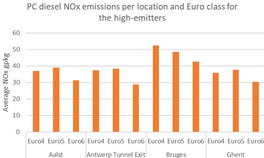
Figure 4-68: High-emitter averages for NOx for diesel cars per test location
