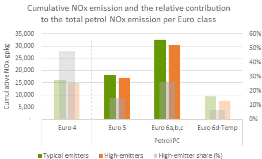
Figure 4-65: Total NOx contribution of the petrol passenger car high and normal range emitters per Euro class (coloured bars, left-hand side Y-axis), and the relative share of high emitters for Euro 4 separately and Euro 5 – 6d-Temp combined (grey bars right-hand side Y-axis)
