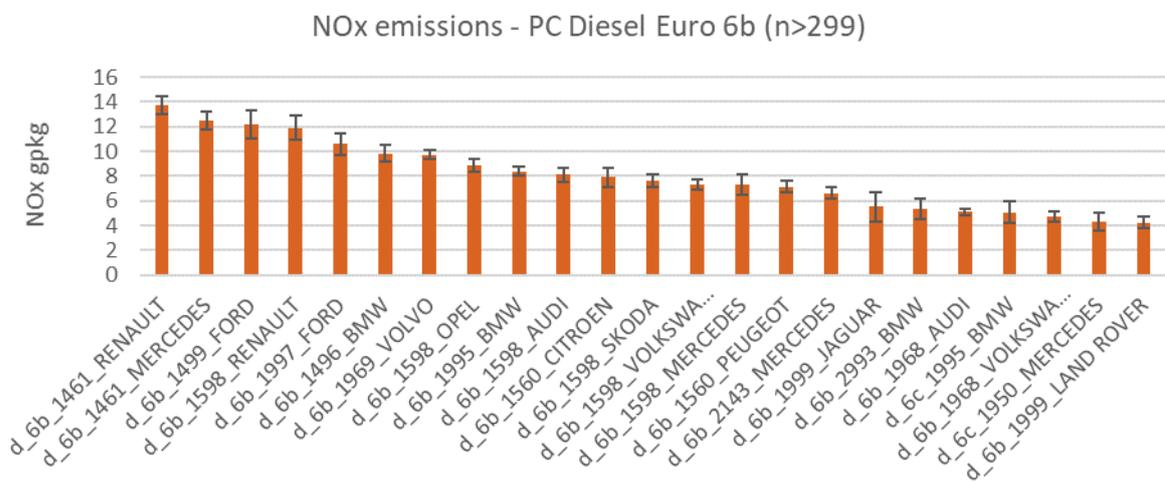
Figure 4-30: Overview of the diesel Euro 6b passenger car NOx emissions per engine type
