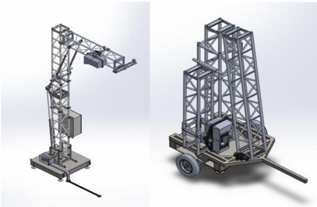
Figure 3-1: The truss system when fully deployed (left) and when stowed back for transport (right)
