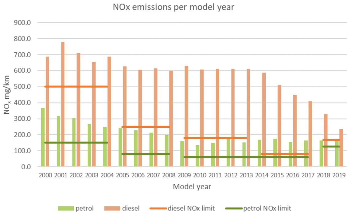
Figure 4-25: Passenger car NOx emission factors in mg/km based on the MILE21 methodology for deriving realistic CO<sub>2</sub> emission factors, per model year and per fuel type for the Flemish dataset. Note that the latest limits take the RDE conformity factor into account.
