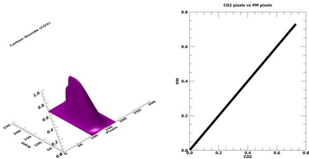
Figure 4-54: An exact plume overlap, resulting in a plot showing one straight line with the slope that equals the ratio of PM/CO<sub>2</sub>
