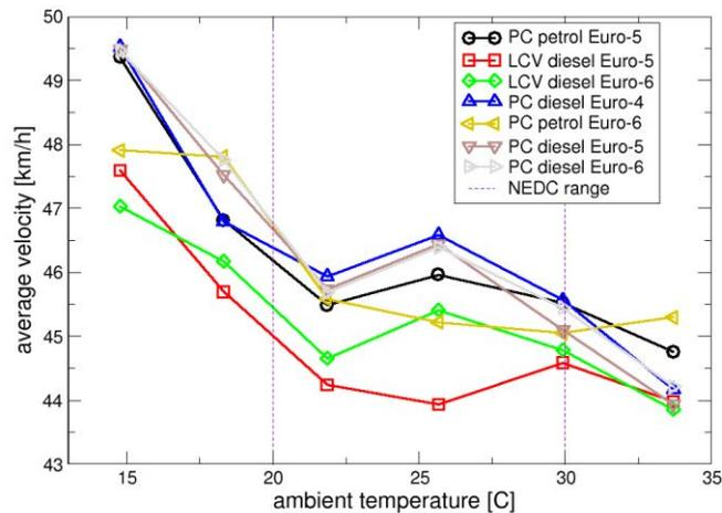
Figure 4-74: Distribution of the Ghent average velocity as a function of the ambient temperature
