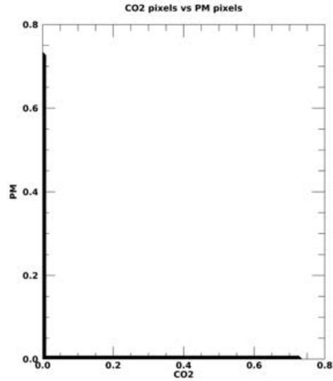
Figure 4-51: These are the plumes coming from the rear of the vehicle. The rear of the vehicle starts at scan 1. The PM plume is on the right-hand side of the car and the CO<sub>2</sub> plume is on the left-hand side. If the CO<sub>2</sub> and the PM come from different sides of the vehicle and do not overlap; the values of the plot are on their perspective axes. This means that the PM emissions do not originate from the exhaust.
