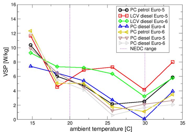
Figure 4-75: Distribution of the Ghent vehicle-specific power as a function of the ambient temperature
