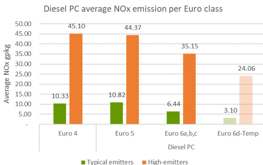
Figure 4-60: Average NOx emission rates in g/kg fuel for normal range and high-emitting diesel passenger cars
