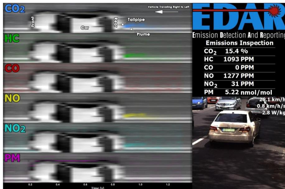
Figure 2-1: An example of a 2D image of a sampled passenger car, combined with the measurement read-out
