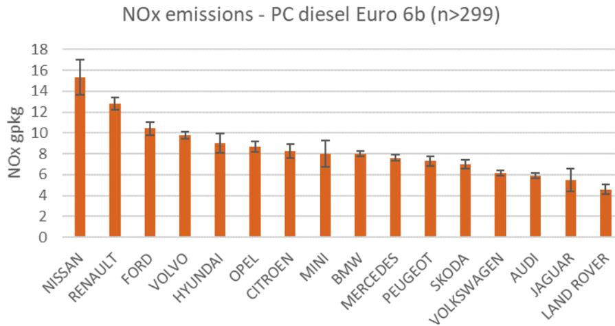
Figure 4-28: Passenger car NOx emissions per manufacturer, diesel Euro 6b
